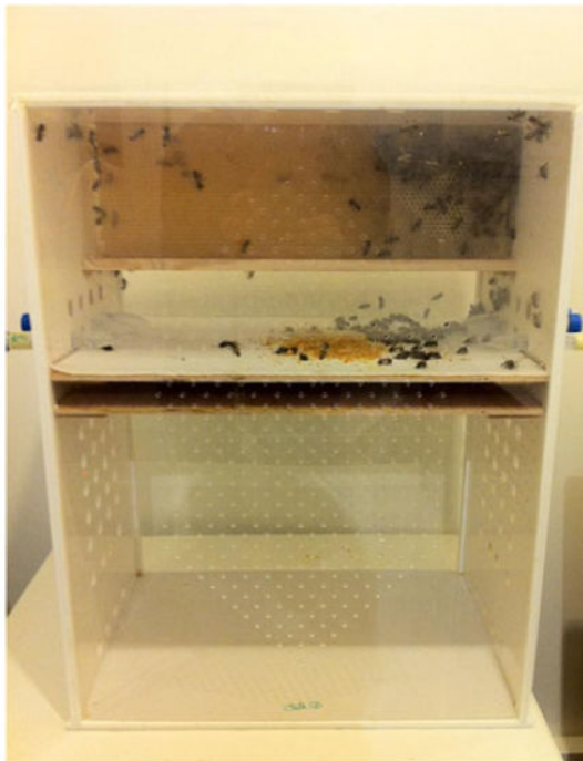
Figure 1. Cage designed to maintain drones under laboratory conditions.
